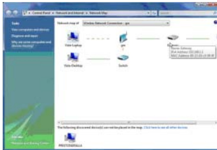
Figure 3. The new Network Map shows you every device on your network and displays details about each, such as IP and MAC addresses.
