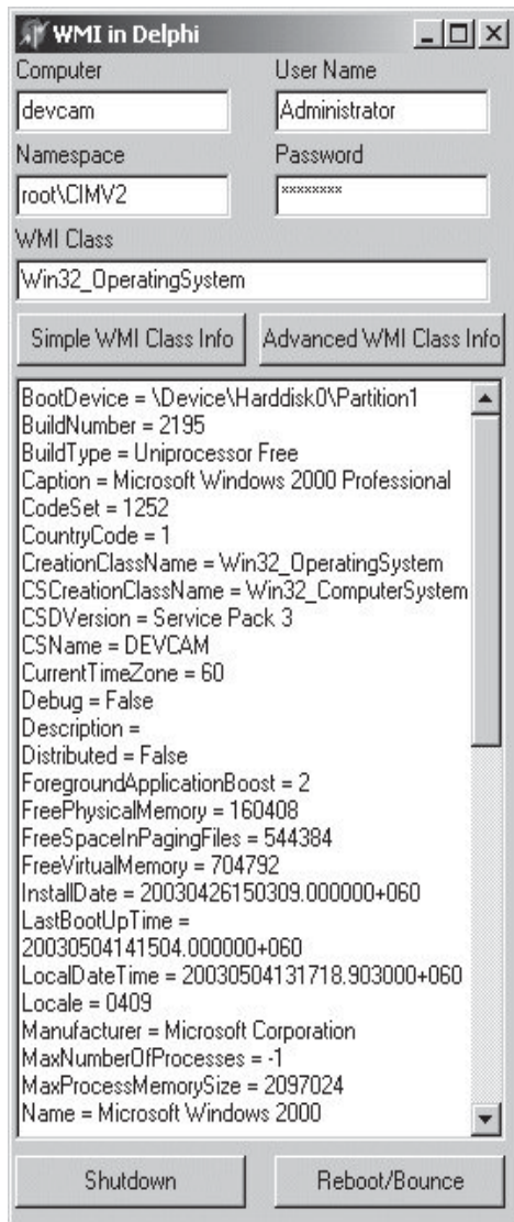
Figure 5 – Using WMI on remote computers
